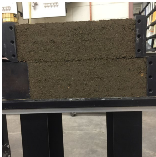
Figure 23. Backfill with geosynthetic inclusion after shearing
