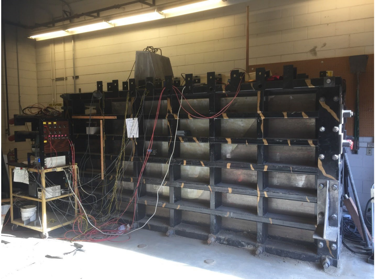
Figure 43. Tiger Cage with T7B-GRSW model test
