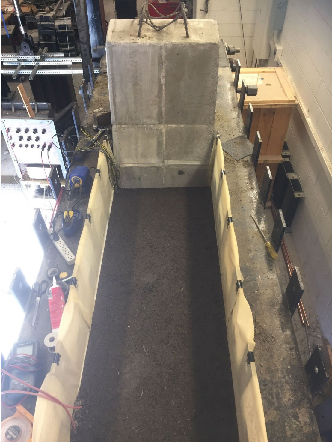
Figure 44. Wall top after soil compaction
